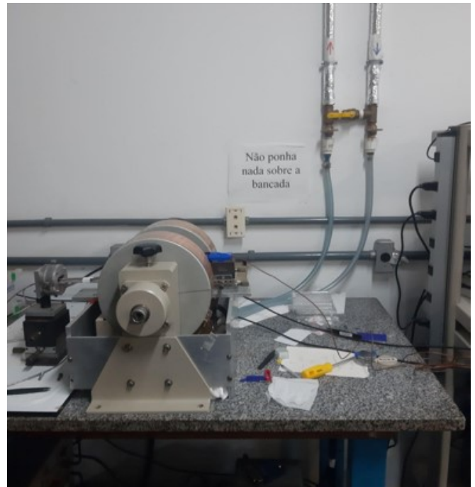
FIG. 19: Image of ferromagnetic resonance (FMR) machine in the laboratory with the water supply connected.
